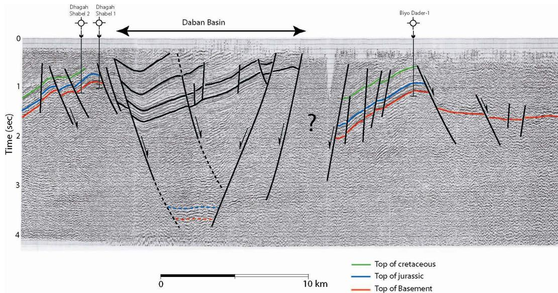
**Fig. 2.** Seismic profile crossing Daban basin, illustrating structural style of the area.
